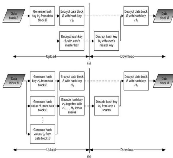
Fig1. Flow diagram of the generation of Dekey
